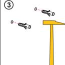
Insert the rawl plugs into the drilled holes.
